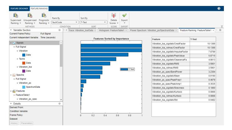
The app operates on data ensembles. An *ensemble* is a collection of data sets, created by measuring or simulating a system under varying conditions. An individual data set representing one system under one set of conditions is a *member*. **Diagnostic Feature Designer** processes all ensemble members when executing one operation.
